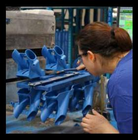
A ceramic mold is created by dipping or "investing" the assembled patterns in liquid ceramic slurry, draining, and then coating with a dry "stucco" sand. After drying, this process is repeated several times until a specified shell thickness results. The ceramic shell ranges in thickness from 3/16" to 1/2" depending on the size of the part being produced.
