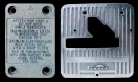
Normally, raised letters or numbers in protective depressed pads are easiest to manufacture. A .020" high character on a depressed pad yields sharp, castable features. Specify exact text and dimensions of the figures. Logos can be investment cast to almost any design.
